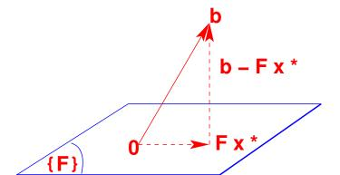
**Illustration of theorem:**  $x^*$  is the best approximation to the vector b from the subspace span $\{F\}$  if and only if  $b - Fx^*$  is  $\bot$  to the whole subspace span $\{F\}$ . This in turn is equivalent to  $F^T(b - Fx^*) = 0 \triangleright$  Normal equations.
