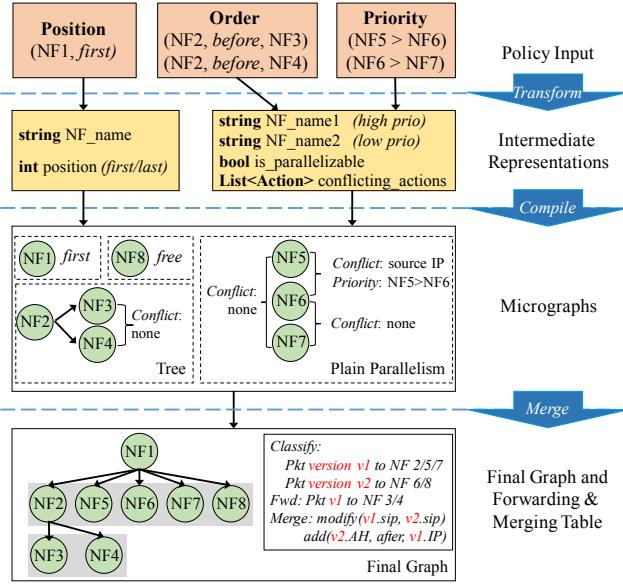
Figure 2: Service Graph Construction Workflow
