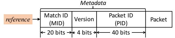
Figure 5: NFP packet data structure
