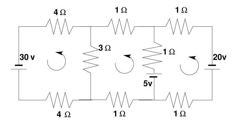
Problem: Determine the loop currents in a an electrical circuit - using Kirchhoff's Law  $(oldsymbol{V}=oldsymbol{R}oldsymbol{I})$
