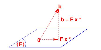
**Illustration of theorem:**  $x^*$  is the best approximation to the vector b from the subspace span $\{F\}$  if and only if  $b - Fx^*$  is  $\bot$  to the whole subspace span $\{F\}$ . This in turn is equivalent to  $F^T(b - Fx^*) = 0 \triangleright$  Normal equations.
