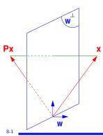
Geometrically,  $\boldsymbol{P} \boldsymbol{x}$  represents a mirror image of x with respect to the hyperplane span $\{w\}^{\perp}$ .
