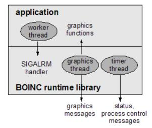
Figure 3: The BOINC runtime system's thread structure
