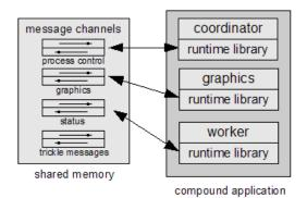
Figure 4: A compound application consists of several processes, each of which handles particular message channels
