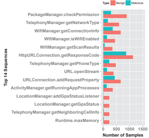
Figure 5: Top 14 differences of sensitive API calls between benign and malicious apps by 3,032 benign and malicious samples
