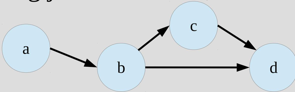
$$\begin{aligned} P(D|a) &= \sum_b \sum_c P(b, c, D|a) \\ &= \alpha \sum_b \sum_c P(a, b, c, D) \\ &= \alpha \sum_b \sum_c P(D|b, c)P(c|b)P(b|a)P(a) \\ &= \alpha P(a) \sum_b P(b|a) \sum_c P(c|b)P(D|b, c) \end{aligned}$$
