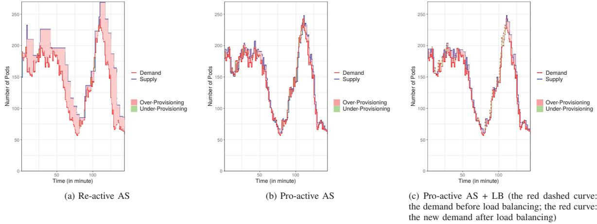
Fig. 5: The scaling behavior of three controllers on EDC#1 ( $avg\_utilization\_thresh= 80\%$ ,  $max\_rejectionRate\_thresh = 1\%$ ).
