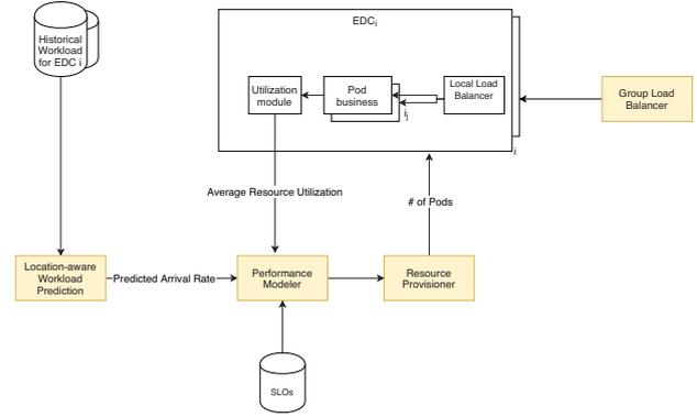
Fig. 2: Components of the proposed group controller.
